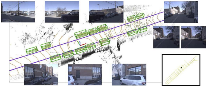
Figure 1: We introduce a dataset for 3D tracking and forecasting with rich maps for autonomous driving. Our dataset contains sequences of LiDAR measurements, 360° RGB video, front-facing stereo (middle-right), and 6-dof localization. All sequences are aligned with maps containing lane center lines (magenta), driveable region (orange), and ground height. Sequences are annotated with 3D cuboid tracks (green). A wider map view is shown in the bottom-right.
