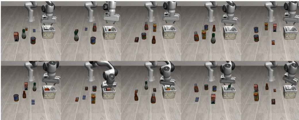
Figure 2: Example environments from the LIBERO-Object benchmark [2]. The robot manipulates household objects according to natural language instructions.
