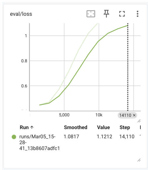
(a) Evaluation loss (increasing trend indicates overfitting).
